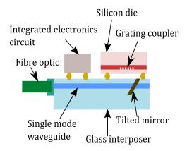
Figure 1 suggested solution to achieve high speed applications
